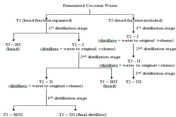
**Figure 1.** Experimental set-up for the distillation of fermented coconut water
